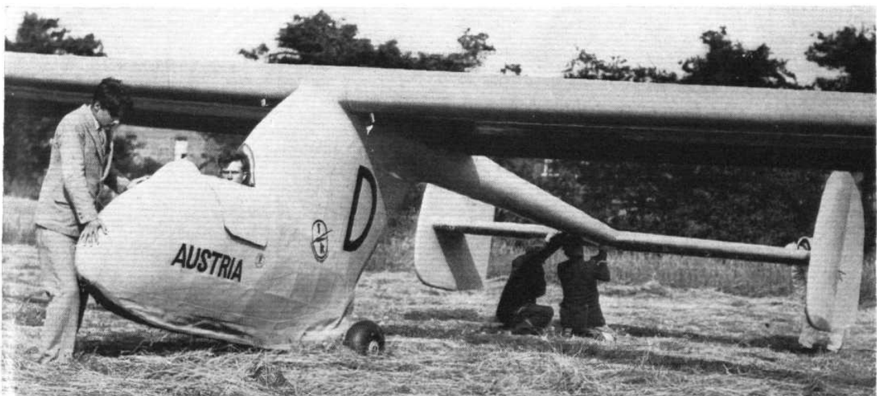
The "Austria" which was built for Herr Kronfeld in the Segelflugzeugwerke at Kassel. The small wheels have recently been added to facilitate towing-off by an aircraft. (FLIGHT Photo.)
